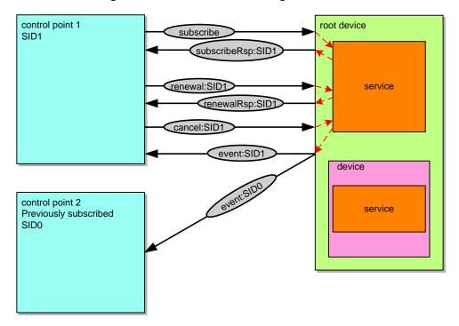
Figure 4-1: — Unicast eventing architecture
