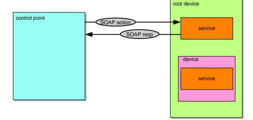
Figure 3-1: — Control architecture
