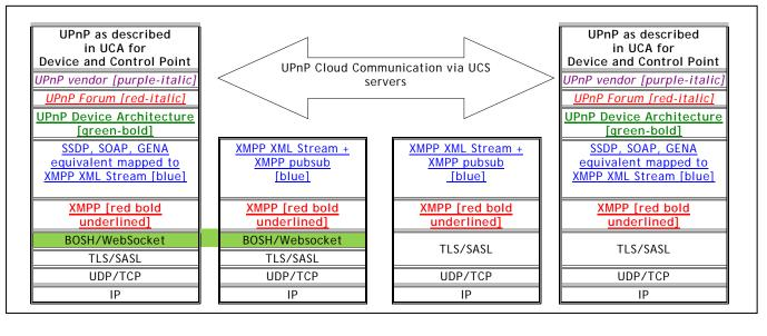
Figure C-12: — BOSH and WebSocket at UCA component stacks
