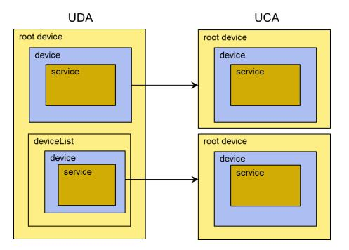
Figure C-7: — UDA to UCA Mapping of embedded devices
